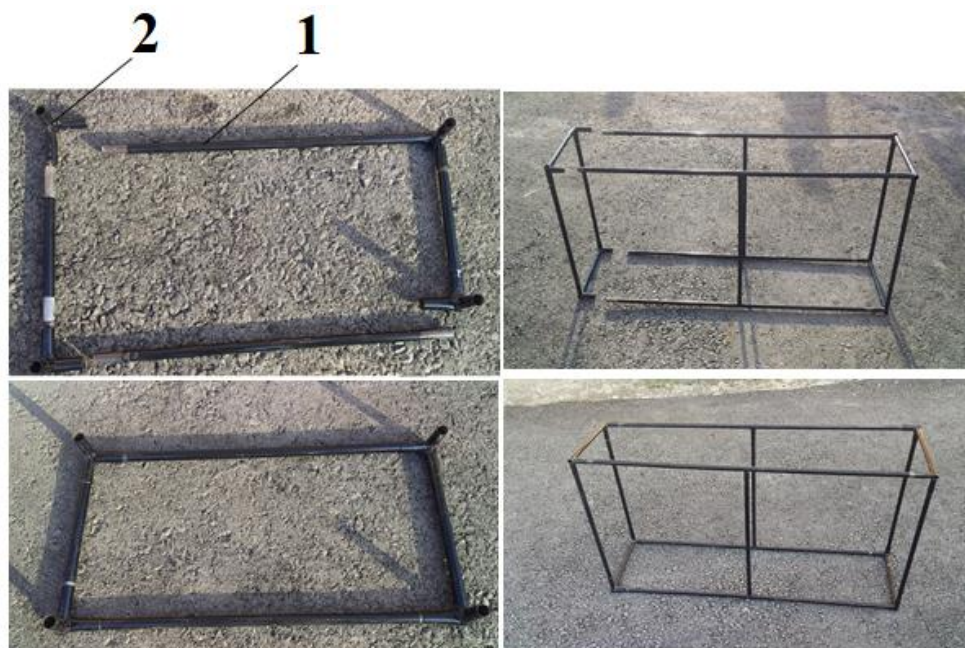
Figure 1. Fragments of assembled parts of the frame of a newly created device for receiving, transporting and storing live cocoons
