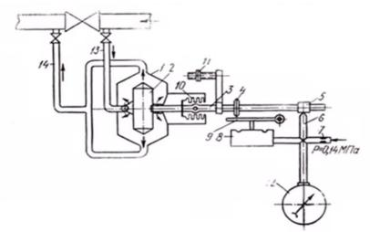
1- scheme of a density meter with a pneumatic switch with a sinking shield.
