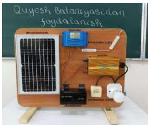
Figure 1. Model showing the process of obtaining electricity from solar energy.
