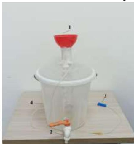
Figure 2. The simplest biogas generator.
