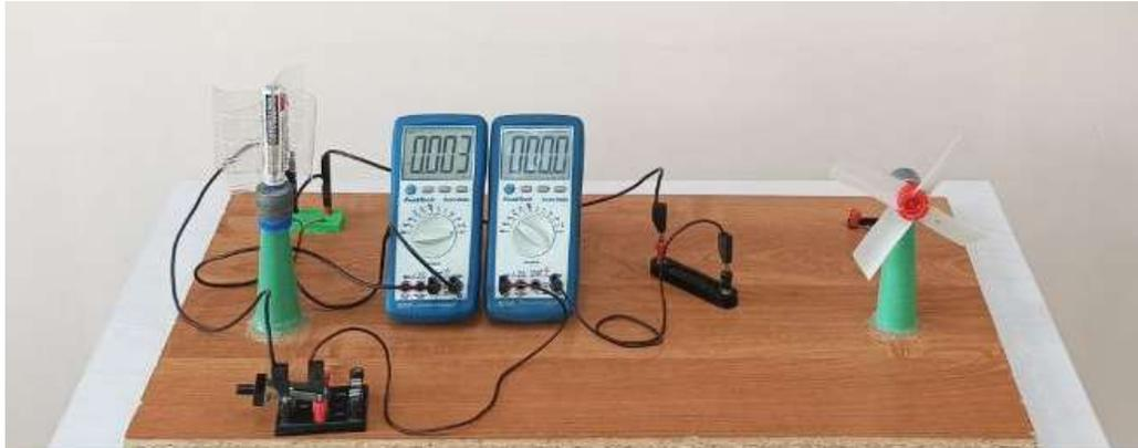
Figure 3. A system of devices representing the mechanism of obtaining electricity from wind energy.
