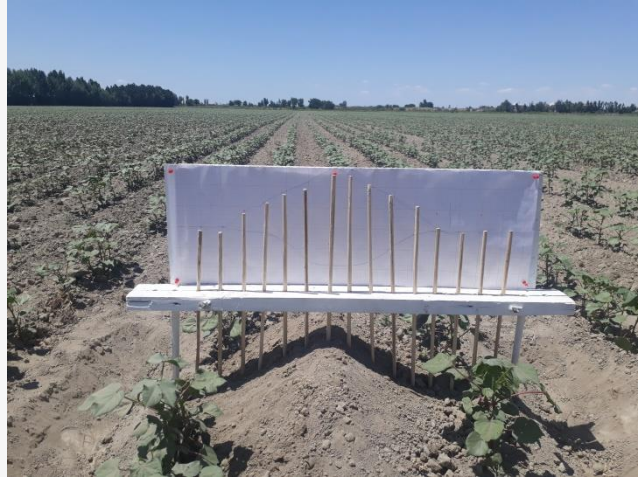
3-picture. Determine the process of pawl profile between cotton rows.
