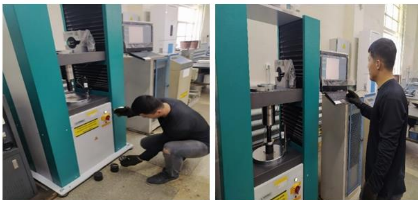
5-rasm. Gidravlik pressda namunani sinovga tayyorlash.
