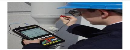
Moving in a homogeneous medium, ultrasonic vibrations do not change their direction. If, for example, there is a crack along the way, some of the waves will be reflected from it, which will be registered by the receiver. The obtained data is displayed on the monitor of the ultrasonic flaw detector. By the time of registration of reflected waves, you can find out where the defect is located and the main characteristics of the latter.
